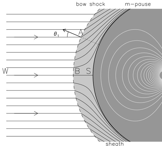
A simplified of the day-side magnetosphere. Flow streamlines are shown as solid curves originating at the Sun, far to the left. The bow shock is a dashed arc and the magnetopause is a thick solid arc. The magnetosphere proper is dark grey, with some white magnetic field lines shown. The magnetosheath is the lighter grey region between the bow shock and the magnetopause.
