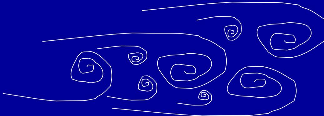
Interacting vortices lead to distortion, stretching, and destruction (spawning).
