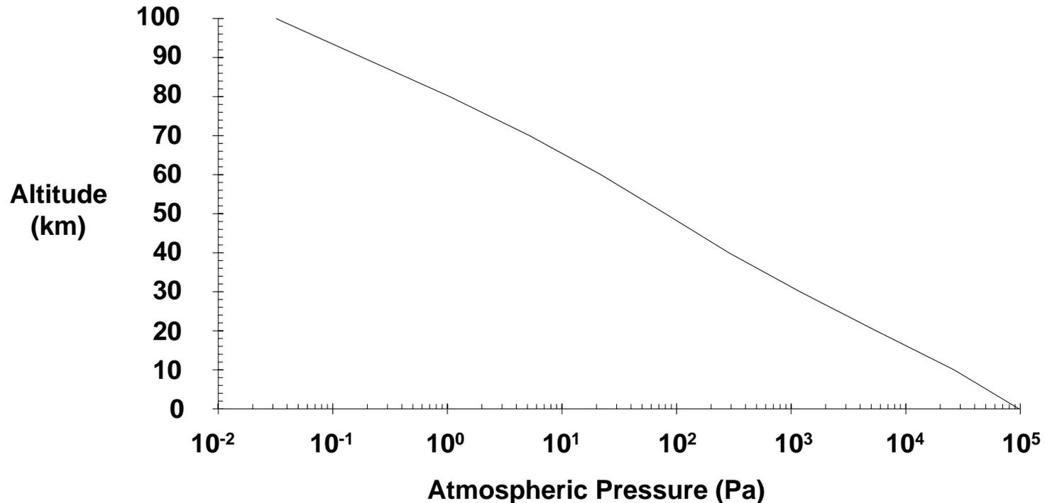
**Spacecraft Must Be Designed to Operate in Extremely Low Pressure Environments**
