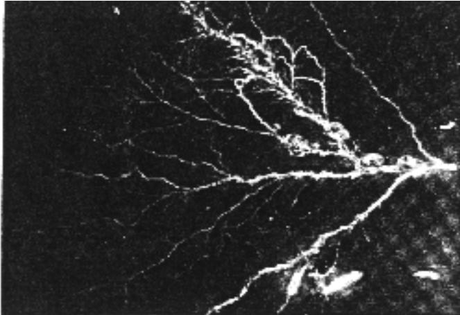
Fig. 1 Optical micrograph of microdamage on a 125- $\mu\text{m}$  silvered FEP Teflon sample irradiated by a 35-keV electron beam.<sup>1</sup>
