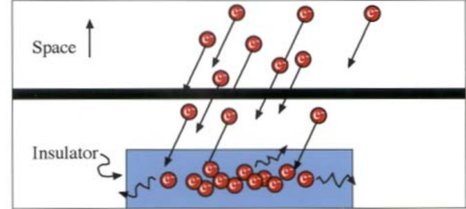
4. Electrons build up faster than they leak off
