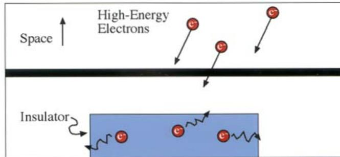
2. Electrons slowly leak out of the insulator
