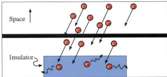
3. Influx of electrons increases to levels higher than the leakage rate
