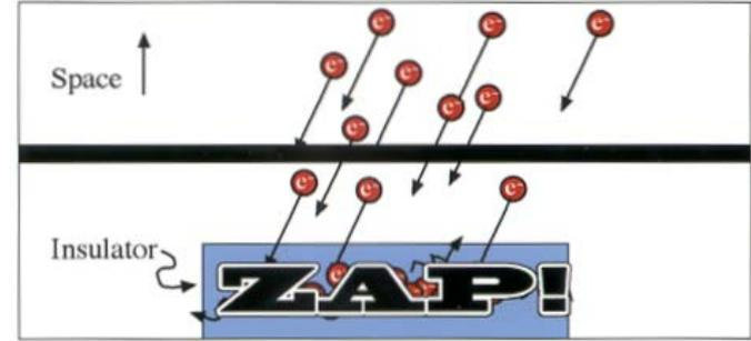
5. Discharge (electrical spark) that damages or destroys the material
