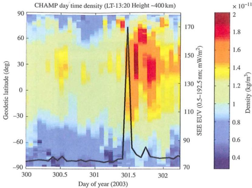
Thermospheric density enhancements measured by accelerometers on the CHAMP satellite (altitude ~400 km) and GRACE satellite (altitude ~490 km) during the October 28, 2003 flare. (Sutton et al., 2006.)
