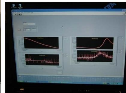
Outputs of spectrophotometer and conductivity meter are digitized and stored on a PC with realtime display via a LabView interface
