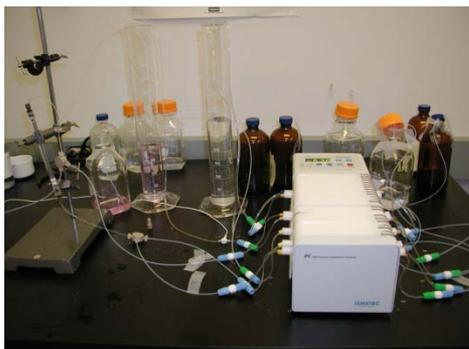
Multichannel peristaltic pump provides throughput. Carrier and reagent is mixed with meltwater for nitrate analysis. Pure portion of melt is diverted to conductivity meter.
