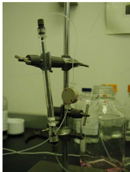
Meltwater with eluents pass through cadmium reaction column before nitrate analysis.
