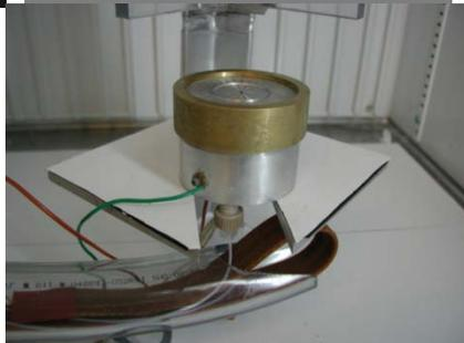
Inner ring melts clean ice; outer ring collects waste water. Capillary slits minimize upward wicking
