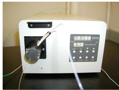
Spectrophotometer measures nitrate concentration in continuous flow at high time cadence with resolution less than 1 ppb
