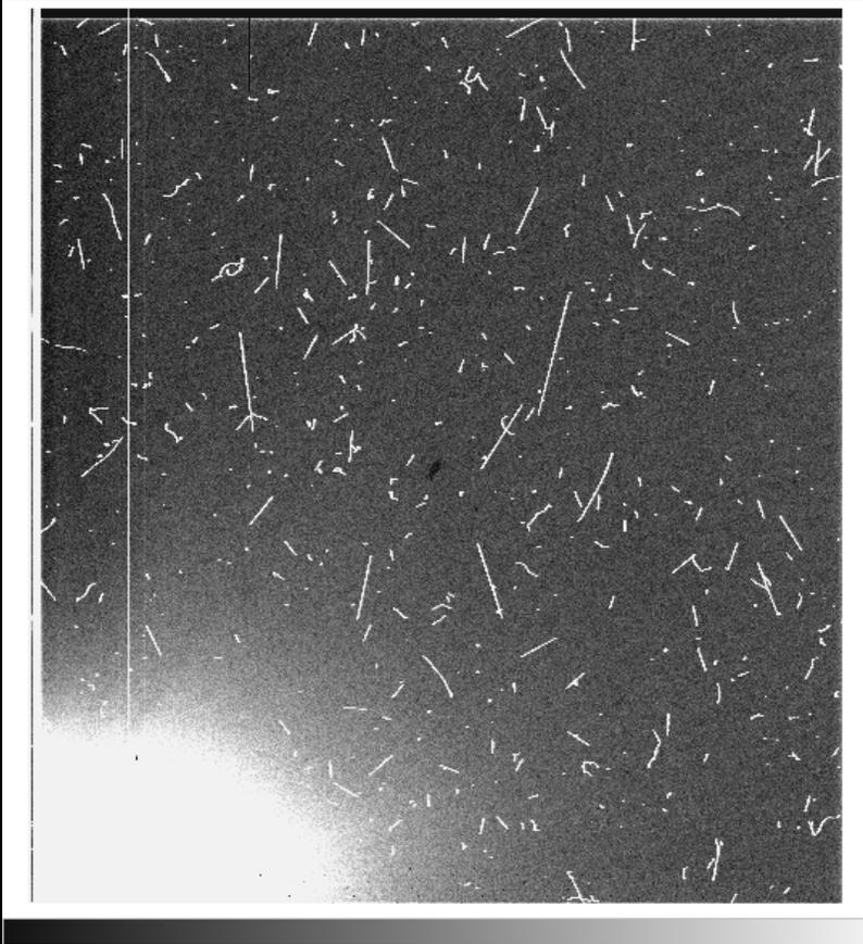
MMT Observatory 1-hour dark frame with GCR tracks
