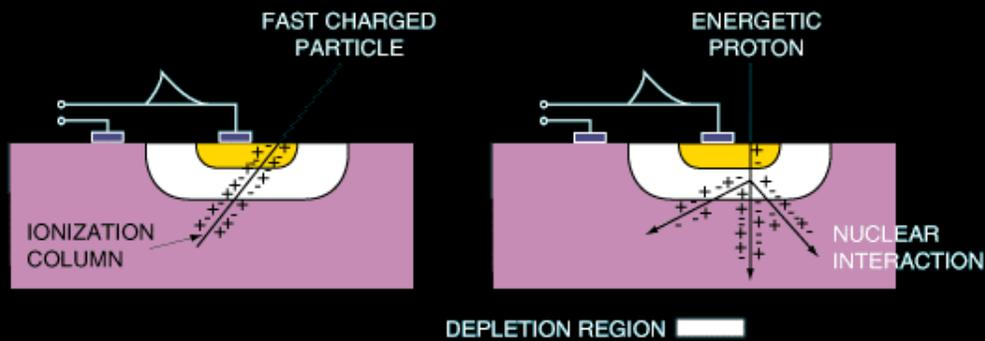
Excess charge causes gate state change
