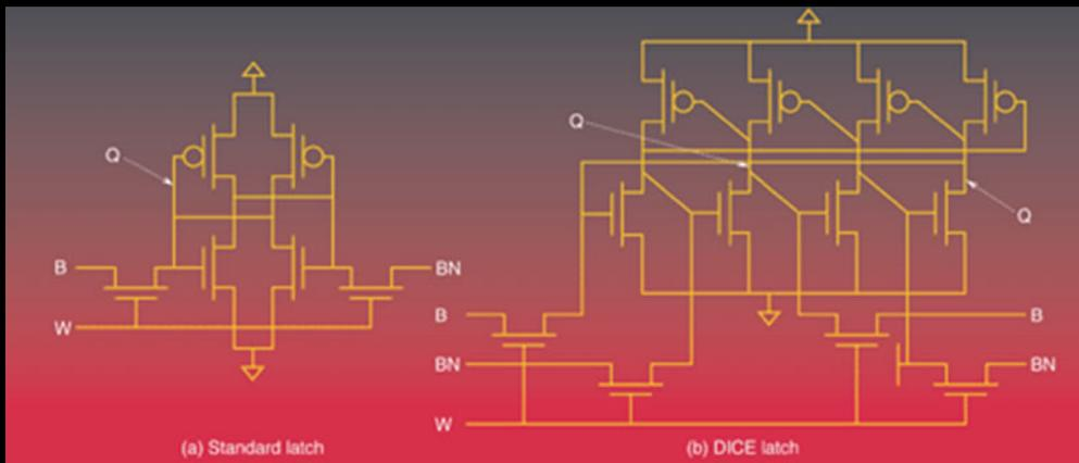
A six-transistor latch, commonly used as the storage element in a static memory circuit, is shown alongside a design-hardened 12-transistor variant.
