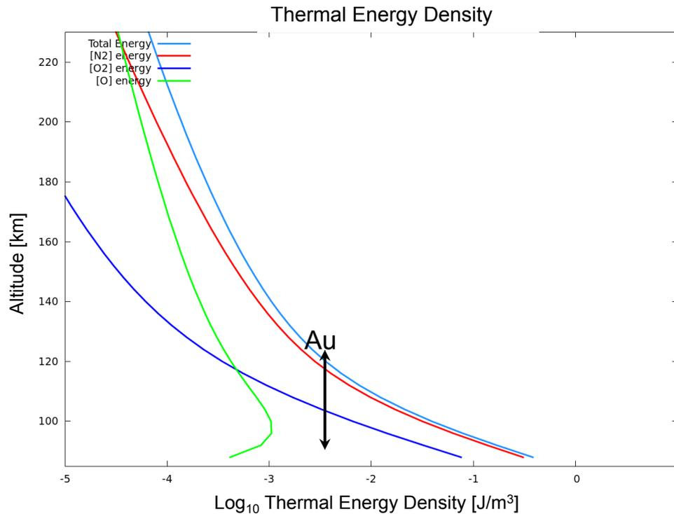
In auroral zone the strong precipitation can result in up to 3 mJ/m<sup>3</sup> between 95 and 120 km altitude.
