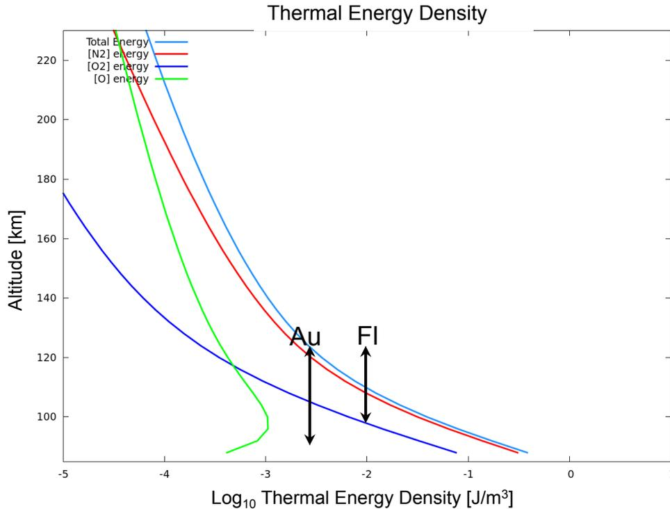
On the dayside a strong X-ray flare can result in up to  $10 \text{ mJ/m}^3$  between 100 and 120 km altitude.
