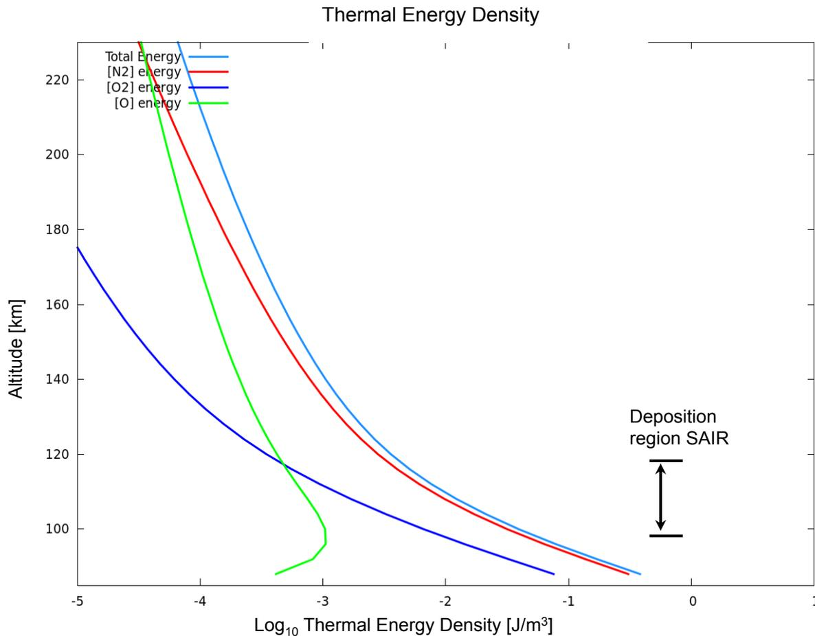
Combining neutral density and temperature produces the altitude distributions of only the thermal energy density.
