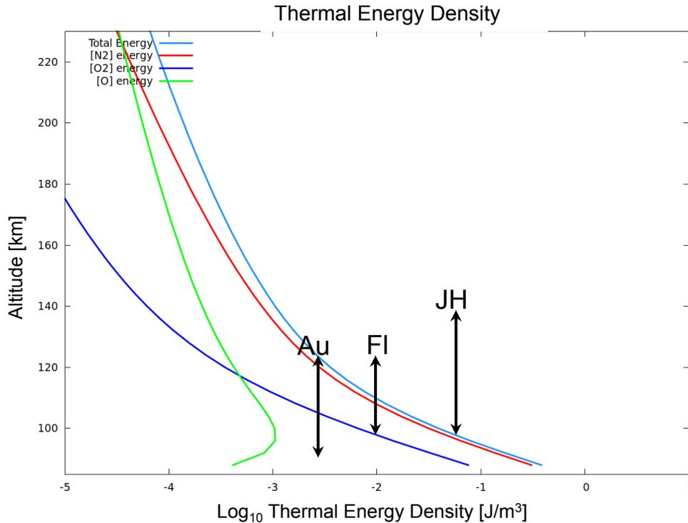
In the auroral zone Joule heating can result in up to 60 mJ/m<sup>3</sup> between 100 and 140 km altitude.
