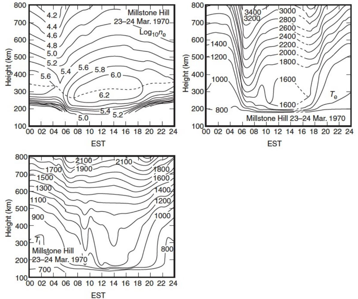
**Figure 11.20** Contours of electron density (top left), electron temperature (top right), and ion temperature (bottom) measured by the Millstone Hill incoherent scatter radar on 23–24 March 1970.<sup>28</sup>  $n_e$  is in  $\text{cm}^{-3}$  and the temperatures are in K.
