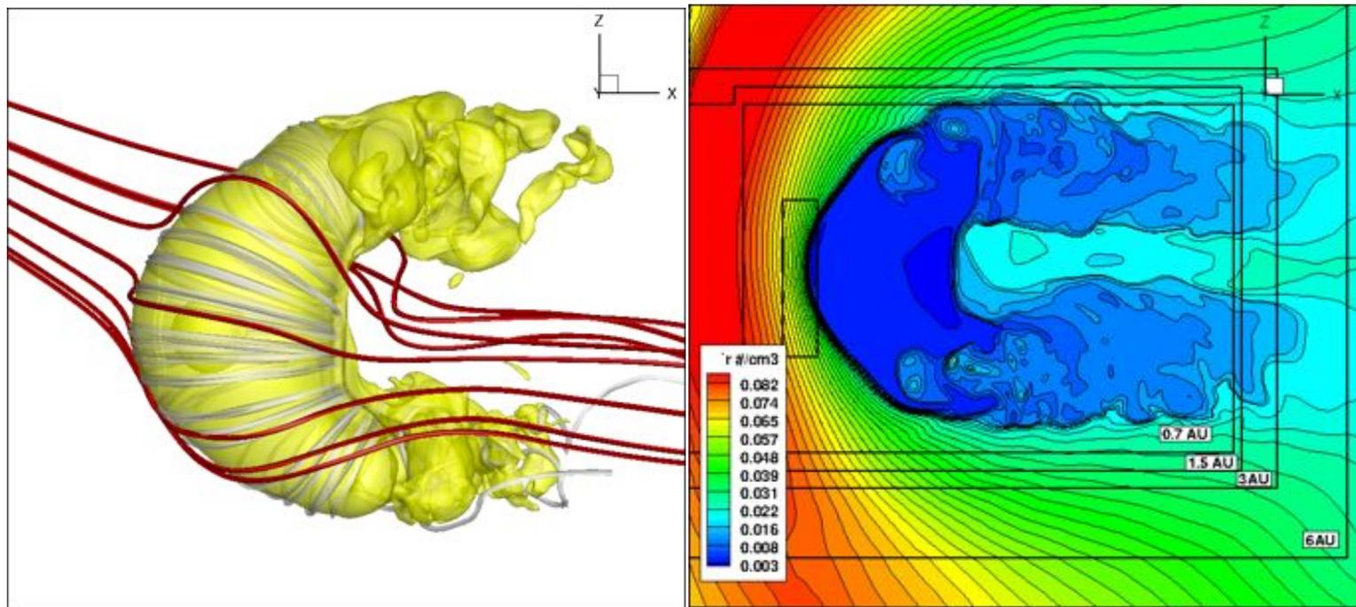
Tension force collimates the heliosheath flow in two jets
