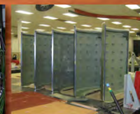
Water Filled Composite Shield Sections
