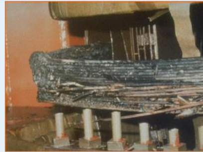
Transformer #5 Lead Overheat
