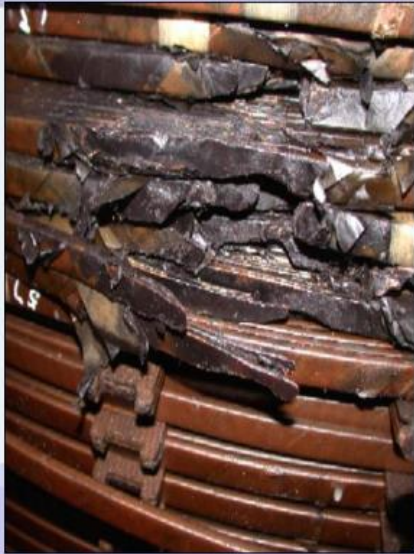
Transformer #4 HV Winding Damage
