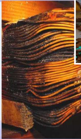
Transformer #5 Lead Overheat
