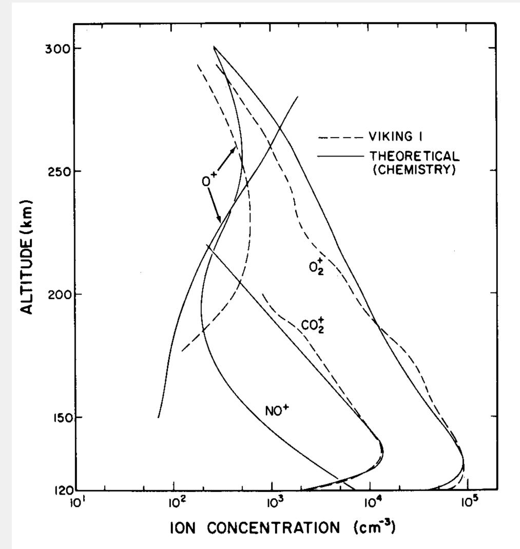
Ion densities for Mars, observed by Viking 1 (dashed lines) and calculated [From HANSON et al. (1977)].
