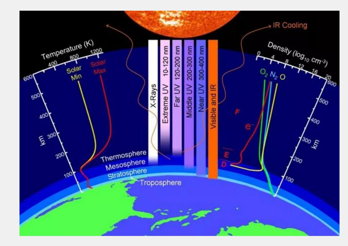
Right: ionization density changes by 100x day vs night, and 10x or more with solar cycle
